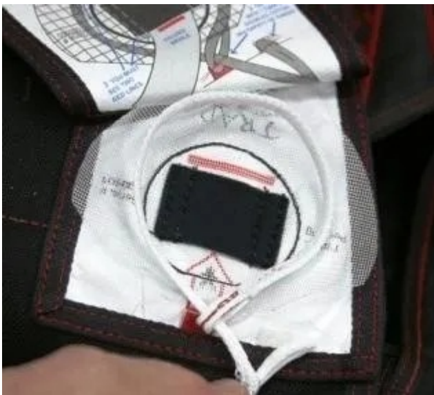
Figur 11: "Trap-linen" gjøres klar for lukking
